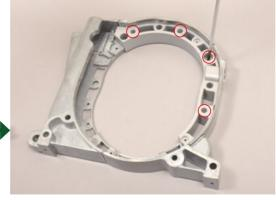
Turn the rotor housing upside down and attach parts F (no. 10 stage 4) and G (no. 7 stage 5).
