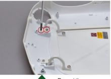
Secure the hinge plate with two of the screws you received with this stage.
