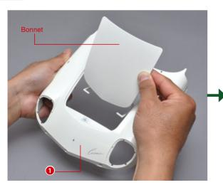
Attach the bonnet you assembled in the previous stage to the front section of the car body (1).
