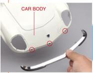
Attach the bumper to the front section of the car body: insert the three linchpins on the bumper into the holes indicated in the photo.
