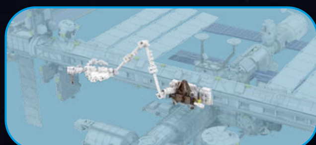
The mobile base system is a platform which moves on a rail along the length of the space station
